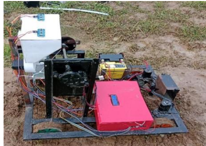
Picture 5. A Prototype Maize Planter with Control of Planting Distance and Seed Quality Based on Size
